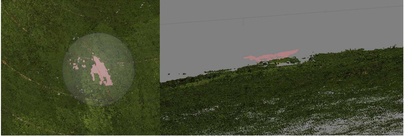
Figure 2. The image on the left depicts the location of erroneous image frames (pink) within a small portion of a center pivot field. The image on the right depicts how these erroneous frames are elevated above the surface of the other image frames for this field.
