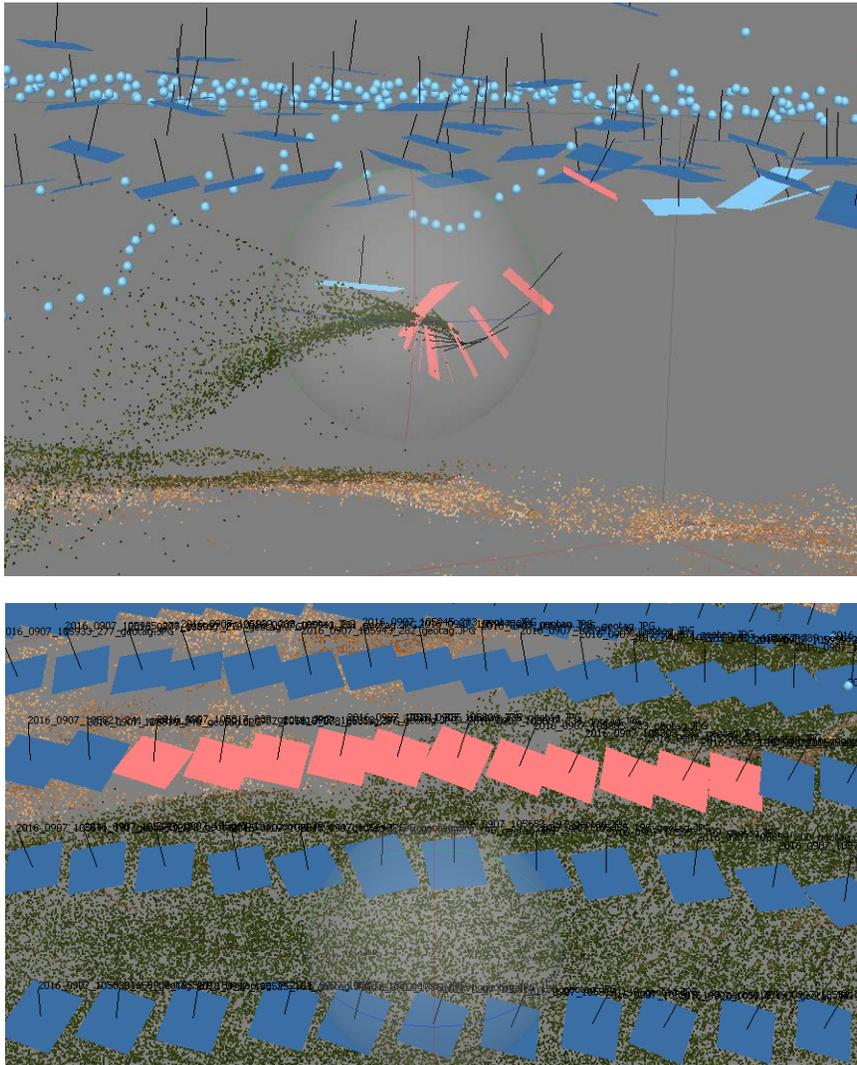
**Figure 1.** The top figure depicts a representation of UAS image frames (blue and pink squares) for which AgiSoft generated erroneous image orientations (orientation is represented by the black lines extending from the image frame) where the erroneous oriented frames are represented by pink squares. The bottom figure depicts the same erroneous image frames (pink squares) after they have been manually corrected.
